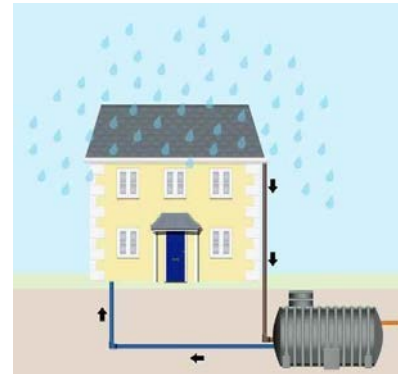
Figure 6 (right): Rainwater harvesting and underground tank
