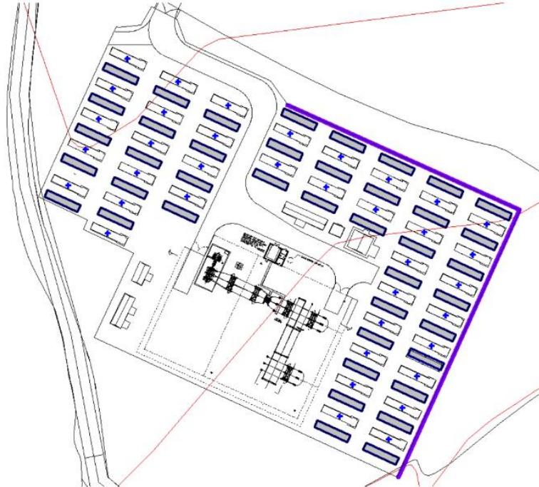
Figure 2 – Extract from Updated Noise Impact Assessment showing the revised location of the Acoustic Fence (Indicated in purple).
