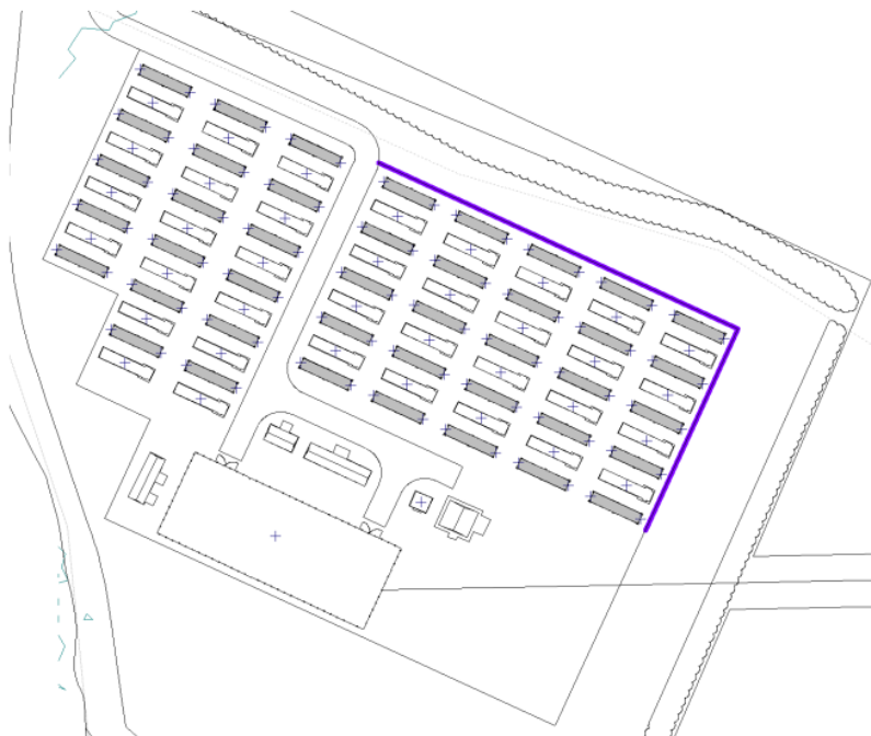
Figure 1 – Extract from Submitted Noise Impact Assessment Showing Initial Location of Acoustic Fence
