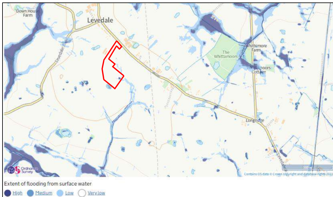
Figure 4.2: Long Term Flood Map – Surface Water Flooding
